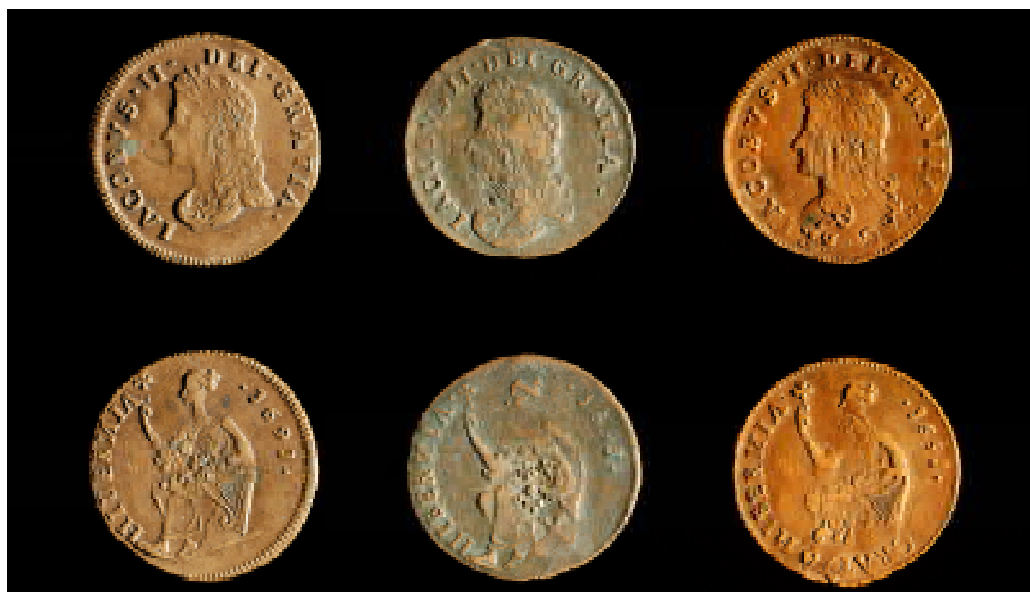
Figure 9 - Weak striking with undertype showing through
