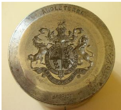
Figure 30 – 32 - French button die with a button it produced displaying the British Royal coat of arms.
