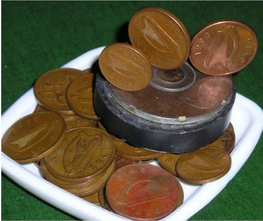
Figure 1 – The figure shows a magnet amongst a tray of 1p and 2p coins from the period 1971 to 1988. These are copper coins, and not being magnetic they remain in the tray unattracted by the magnet. Attached to the upperside of the magnet is a copper-plated steel 1p and two 2p coins. In the centre of these three steel coins is a 1988 2p specimen which, by conventional wisdom, should still be in the tray.
